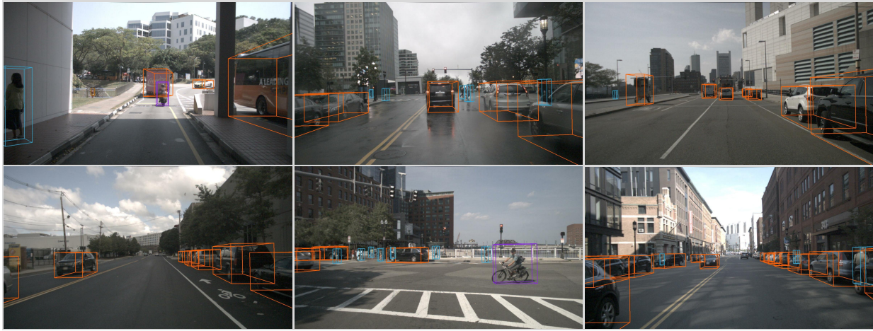
Fig. 3. Visualization of the detection results of MVS3D-pre-trained FCOS3D on the nuScenes test dataset.
